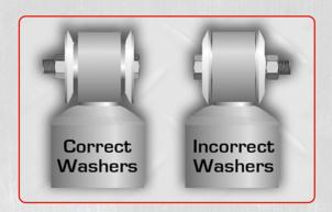
If over compressed, the bushings will restrict the movement of the shock absorber with the articulation of the suspension and put excessive side-loading on it. This restricted movement (side loading) will cause premature rod seal failure, resulting in oil leakage or metal fatigue to the shock absorber end mount.
