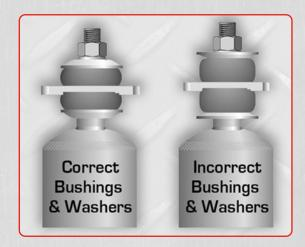
3. The fasteners should be tightened until the bushing expands (bulges) to the same outside diameter of the metal washer (see below). This allows for the proper amount of bushing squeeze so that the shock absorber can move properly in any direction.
