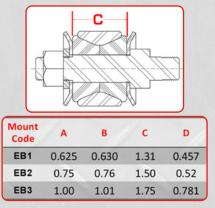
2. Be sure to note the orientation of the washers and the size of inside diameter (D).
