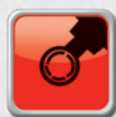
Upper or lower bushing torn
